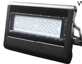
VVDLFL250 - 120 LEDs - 250W - 27,500 Lm - 8.4A 14.4"(H) x 21.5"(W) x 3.6"(D) - 18.7 Lbs
