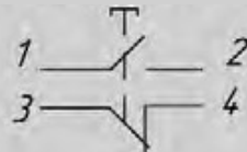
Electric circuit of the button
