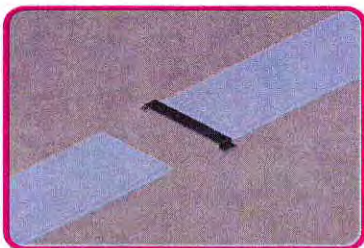
Trunking connection with coupler
